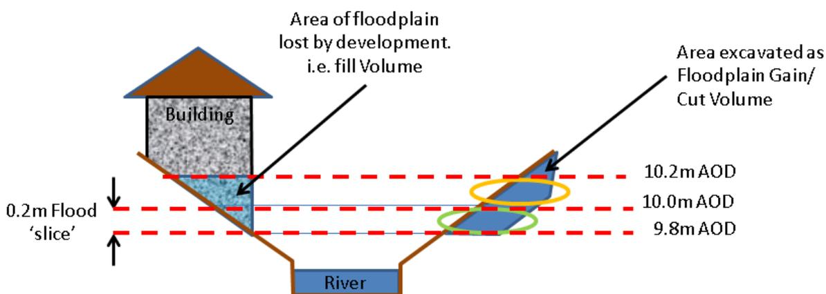
**Figure 3** (above) shows an example of how to calculate what volume of flood water is displaced by a new building in the floodplain and what volume is being provided by the compensation area.
