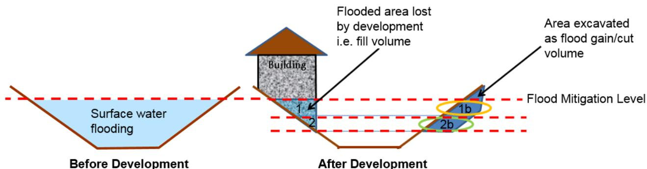
**Figure h)** left show an example of level for level and volume for volume compensation. The volume of ground excavated at a particular elevation is the same or bigger than the corresponding infilled volume i.e. the volume excavated from area 1b is at least equal to the area infilled in area 1. The same is true for area 2b compared to area 2.
