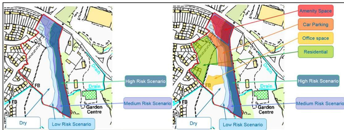
Figure e) left shows an example of how to layout a site to minimise the impact of flooding on the site.
