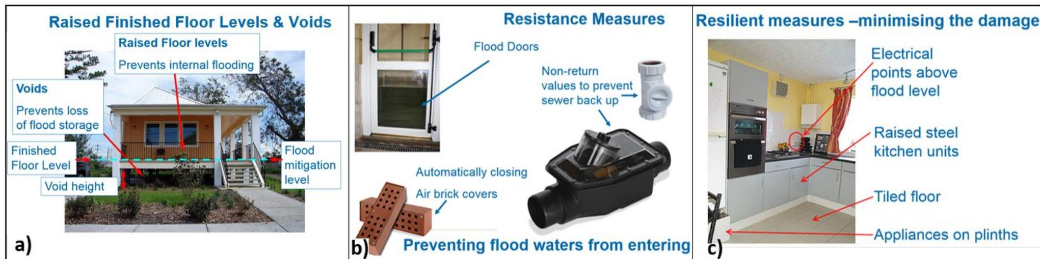
**Figure a)** shows a house with raised finished floor levels and voids. **Figure b)** shows some examples of resistance measures. **Figure c)** show examples of some types of resilient measures.
