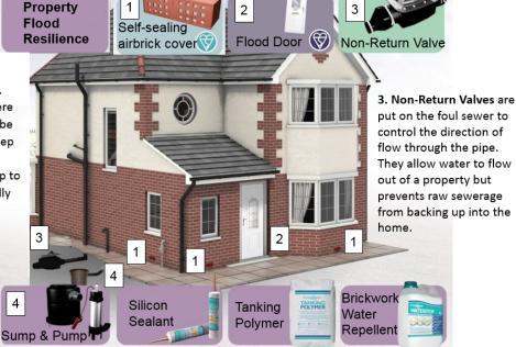
Silicon sealant, tanking polymer and brickwork water repellent. These are special chemical sealants that can be applied to the outside of the house to reduce seepage through the walls. The silicon sealant is used to seal around pipes or wires that run through the wall which can otherwise provide pathways for water to enter a property.
